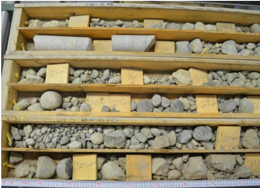
Figure 14 Photo of the uppermost Bcm (clast-supported, massive boulders) and Gm (clast-supported, massive gravel) lithofacies unit of core VTH2014-09, at a depth of 0-33.5m. Lithofacies code from Evans and Benn (2004).
