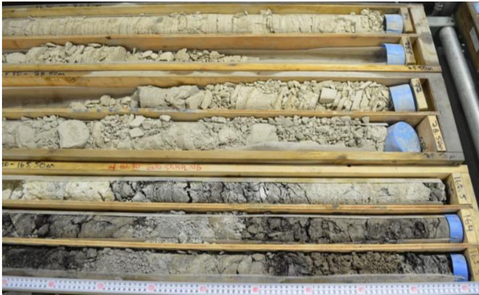
Figure 6 Photo of an S1 (sand with horizontal and draped laminations) lithofacies unit and coal lenses of core VTH2014-06, at a depth of 72.5-165.5m. Lithofacies code from Evans and Benn (2004).
