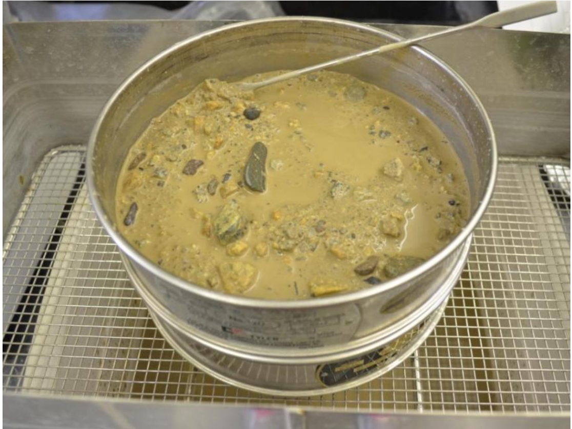
Figure 7 Wet sieving was done on the disaggregated samples.
