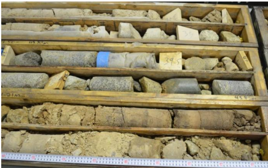
Figure 7 Photo of S m (massive sand) and B cm (clast supported, massive boulders) lithofacies units of core VTH2014-06, at a depth of 29.1-46.5m. Lithofacies code from Evans and Benn (2004).
