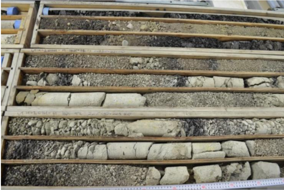
Figure 8 Photo of coal lenses in Flv (finely laminated silts and clays with rhythmites) lithofacies unit of core VTH2014-09, at a depth of 212.0-225.5m. Lithofacies code from Evans and Benn (2004).
