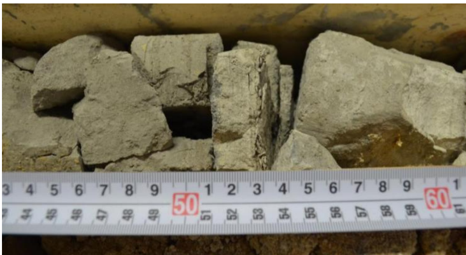
Figure 2b Close up photo of an FI (finely laminated silts and clays) lithofacies unit of core VTH2014-03, at a depth of about 34m. Lithofacies code from Evans and Benn (2004).
